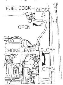
Figure 4. Fuel Cock and Choke Lever
